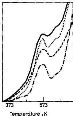
Fig. 2 Trend of the TPR-1 profiles along the catalytic bed U_1 —; U_2 .....; U_4 — — —; U_6 — . — . — . — ;
